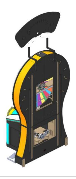
STEP 8: ATTACH HAT BRACKETS TO MARQUEE WITH 8X #8-32 X .375L SCREWS
