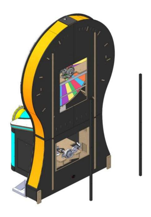
STEP 6: INSTALL SUPPORT TUBES WITH 14X 1/4-20 X 2.00L SCREWS
