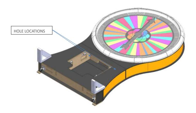
STEP2: PUSH BASE AND DIAL TOGETHER, INSTALL 4 X 5/16-18 X 2.000L SCREWS AND WASHERS THRU HOLES IN BASE UP IN TO DIAL
