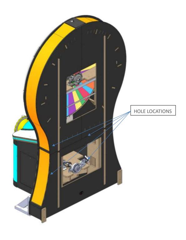
STEP 5: INSTALL CONSOLE WITH 4X 5/16-18 X .500L HEX BOLTS
